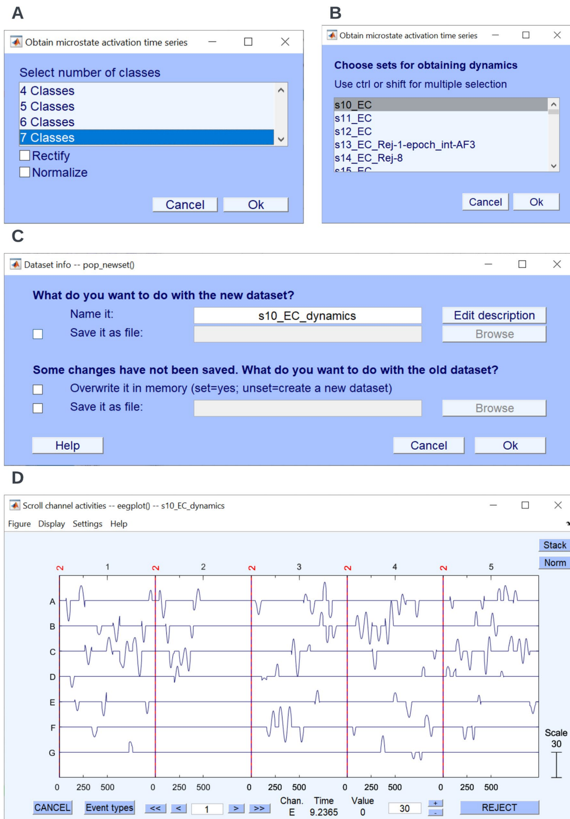
Fig. 13 Timeseries of the fit of individual microstate classes with the EEG data. The time series of spatial correlations of individual microstate classes can be obtained using the menu option Tools → MICROSTATELAB → Obtain microstate activation time
