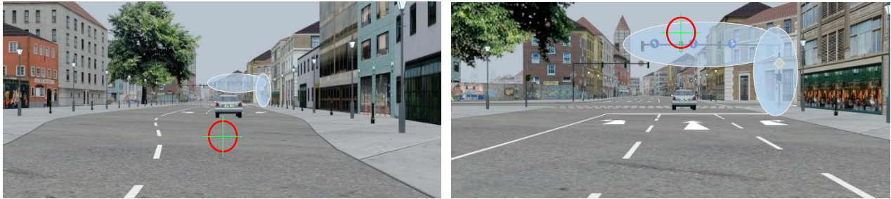
Figure 2. Screenshots of the traffic light as area of interest (white circles) from two different distances when approaching the intersection. The green cross with the red circle depicts the eye position as recorded by the eye tracker.
