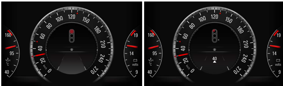
Figure 2. HMI versions as used in the experiment. The simple version showed the current traffic light phase (left). The complex version showed dynamic information on the traffic light phase duration by changes in the filling of the respective color, phase at arrival, action and speed recommendations (right).
